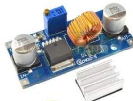
XL4015 MODULE WITH HEATSINK I/P:- 5V-38V O/P:- 1.25V- 36V / 5A
