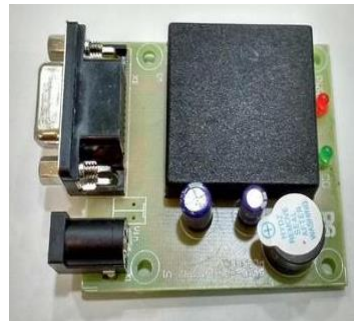
RFID EM18 125KHz RS232 Output
